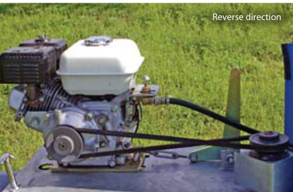
Simple over center lever is used to loosen the v-belt to reverse operating direction.
