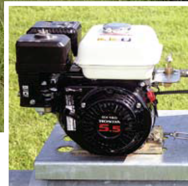
The 5.5 hp Honda engine drive provides a cost effective mechanized irrigation option.
